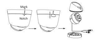
2.4. Fix the mounting base to the ceiling with supplied screws
